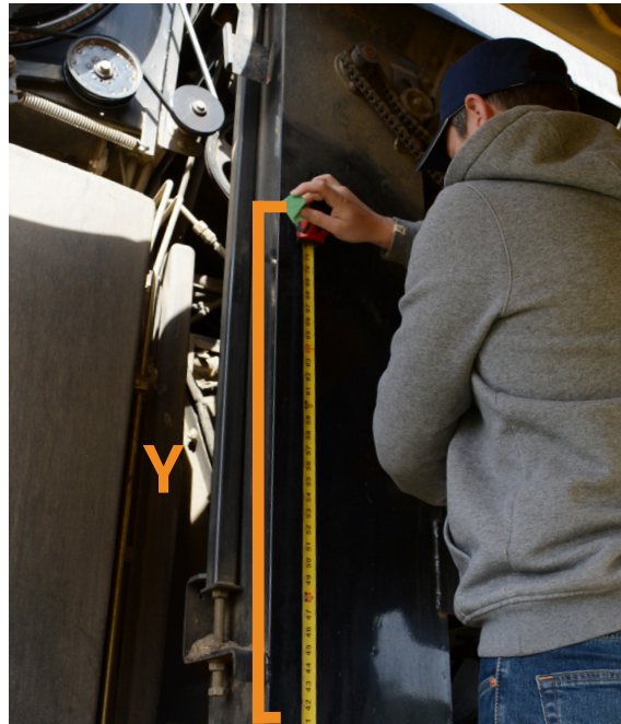
Height (Y) from the center of the bearing to the center of the drill hole
