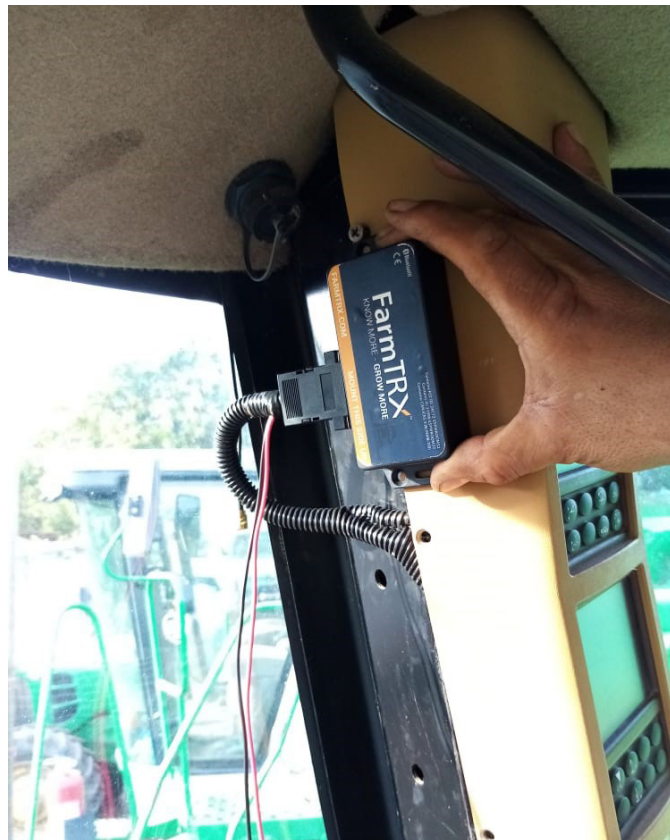
Yield Monitor installed in user-chosen location
