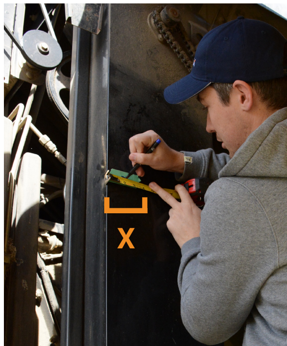
Distance (X) from the back of the clean grain elevator to the center of the drill hole
