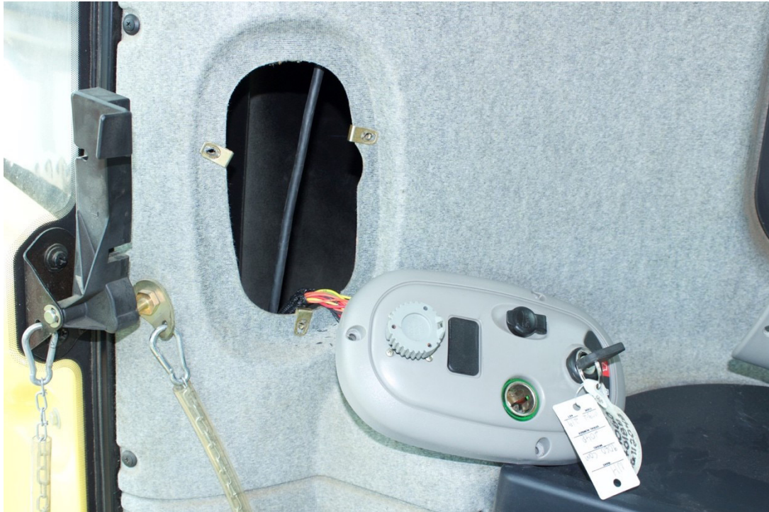
Routing of Primary Wiring Harness along inside of door post with ignition switch assembly removed for access
