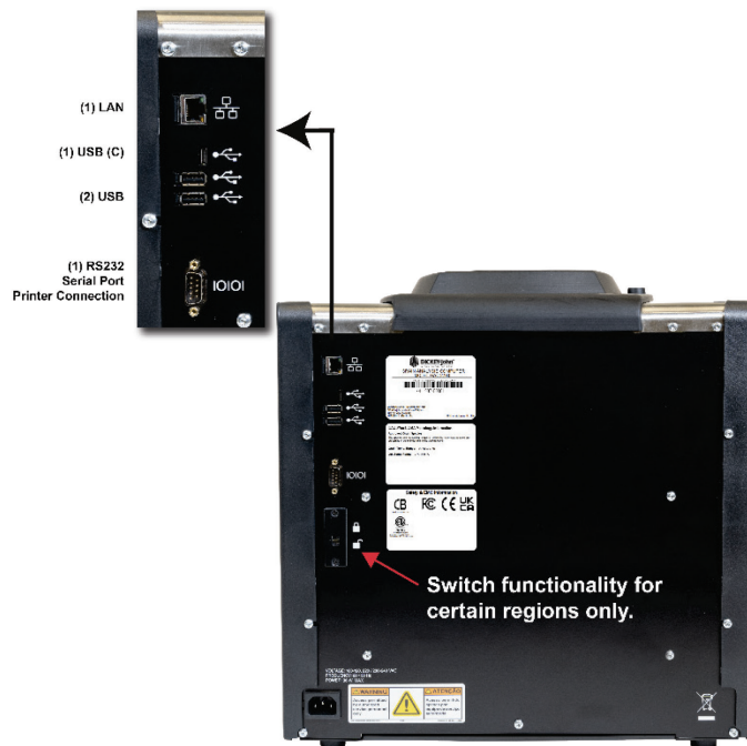
Figure 2 External Communication Connections (Back of Unit)
