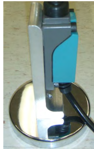
Figure 3: Magnet bolted to short side of bracket.
