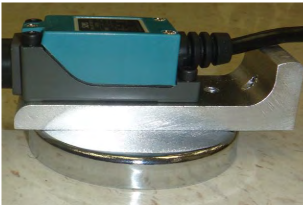
Figure 2: Magnet bolted to long side of bracket.
