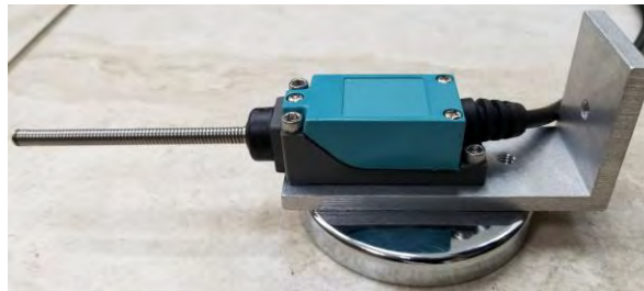
Figure 1: Whisker switch mounted on aluminum bracket.
