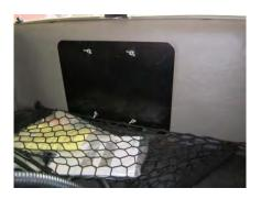
Step 2: Slide the NAV II box off of the threaded studs to expose the connectors on its right side. There is a 12-pin Deutsch plug labeled "Controller Diagnostics."
