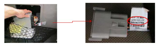
Step 3: Connect the 12-pin Deutsch connector on the AE3380 CIH/Trimble GPS Adapter to the 12-pin Deutsch "Controller Diagnostics". Connect the DB9 to the "RS232" port on the GS2/3 tractor harness.
